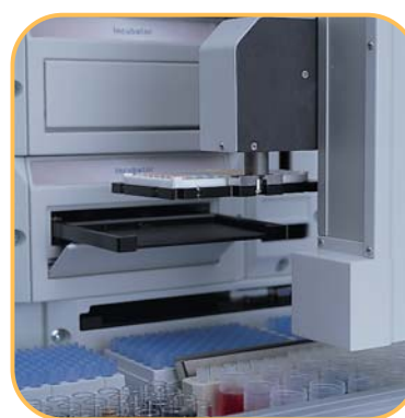
The DSX robotic arm moves microplates and pipettes all sample and reagents.
